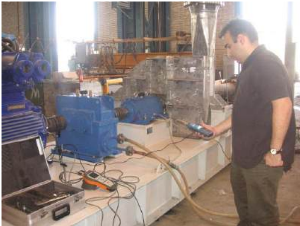
Shop mechanical running & noise test
