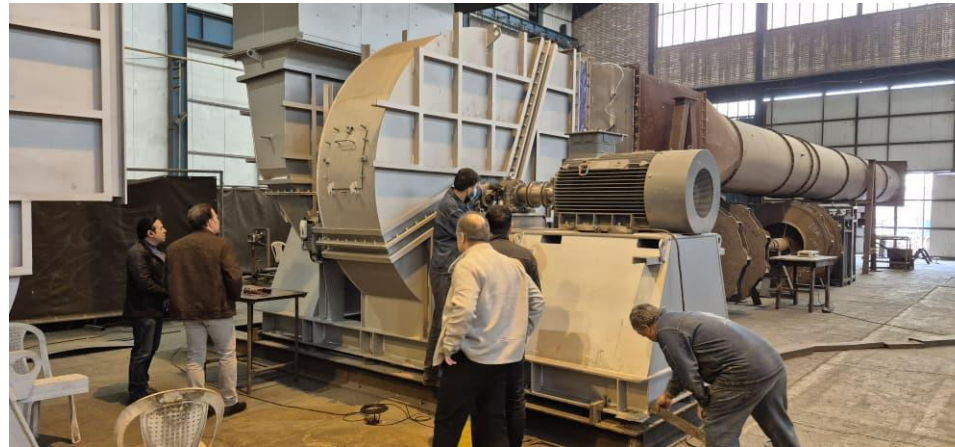
MANGAN SHOP PERFORMANCE TEST
